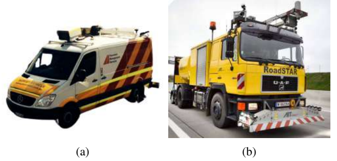
Fig. 1. Survey vehicles used for high-precision road measurements including IRI: (a) ARAN LCMS from Pavement Management Services [3], and (b) RoadSTAR from AIT [4].
